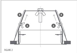
**4.** Loosen the two wing bolts **A** again and move the two attachment plates **B** downwards to secure the fire dome to the false ceiling (as shown in figure 3). When this operation is completed, re-tighten the two wing bolts **A**.
